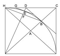
The next step is to find the length of CD. This is done using the similarity of triangles HAC and DBC. This similarity can be seen as both are 45-45-90 triangles. Using the similarity of these two triangles, the following equation follows:
