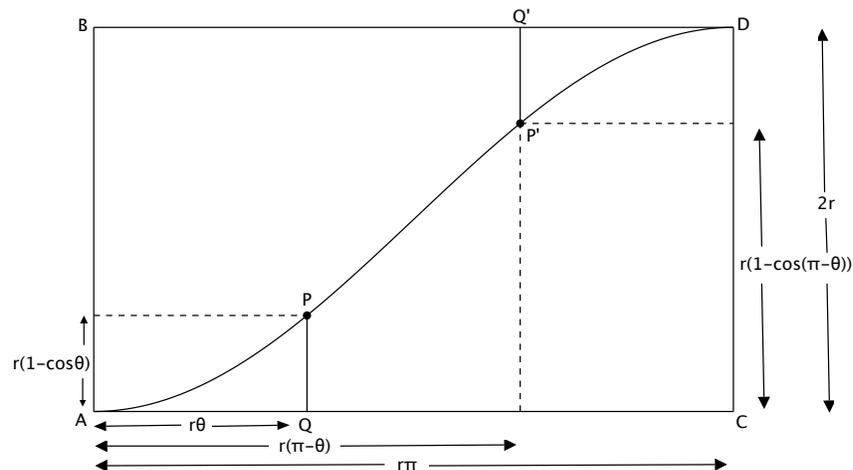
Figure 12; equating the areas above and below the companion curve
